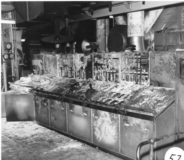
*The fire destroyed the control console located in the engine room. This caused the vessel to drift uncontrolled for some 30 miles before being taken*
